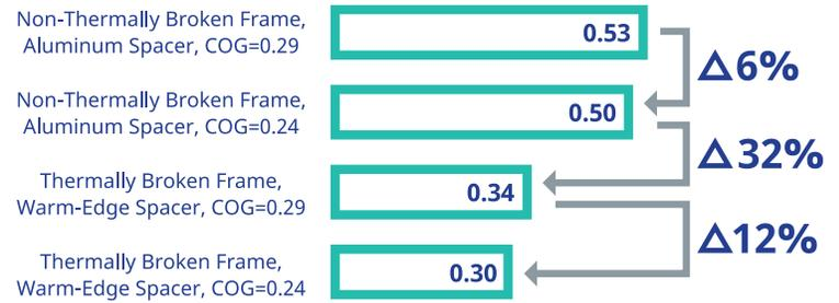
Above — Whole fenestration U-factor as a function of center of glass (COG), edge of glass (EOG) and frame thermal performance.
