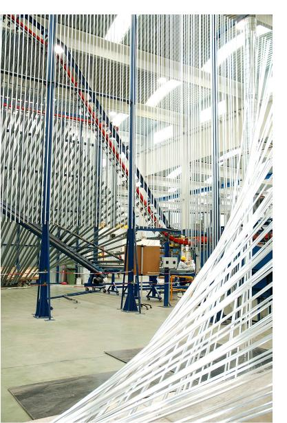
Polyamide is an excellent component since it keeps all its properties intact after going through the standard electrical powder coating process. Thanks to its low conductivity, it is the perfect material for the thermal break in windows, doors and facades, although sometimes it can be challenging due to the electrostatic deposition of powder paint.
